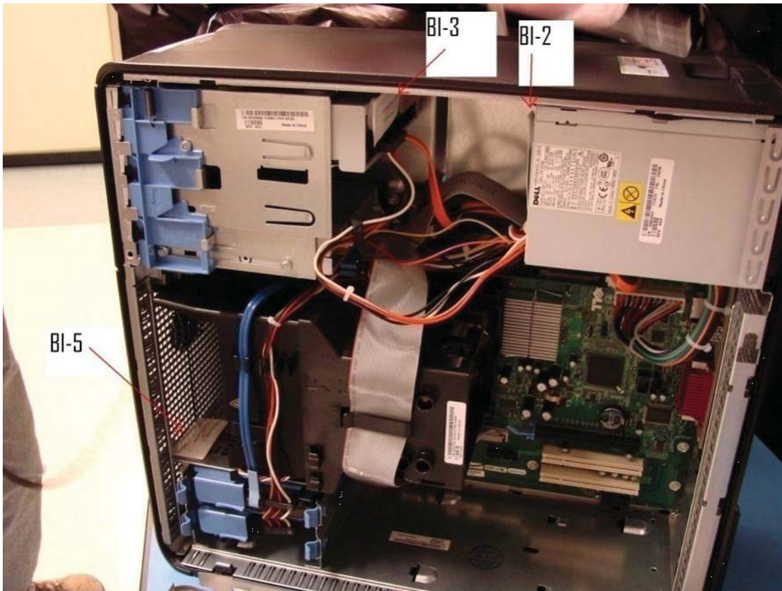
Figure 6-2. Location of the remaining three BIs in both high and low air flow locations inside the computer.
