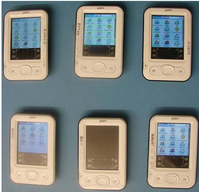
Figure 4-5. PDAs powered on 12 months after exposure.
