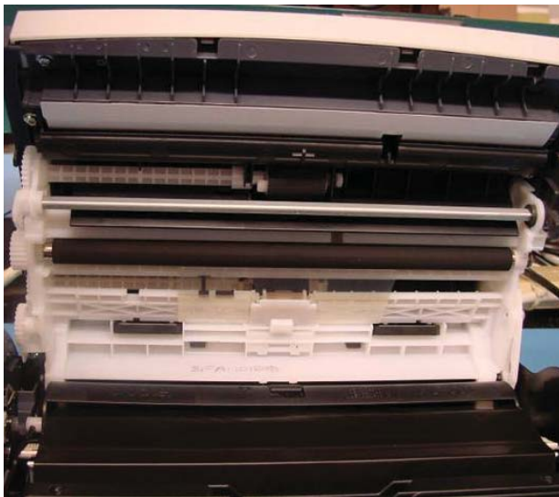
Figure 4-3. Internal view of fax machine 12 months after HPV exposure.
