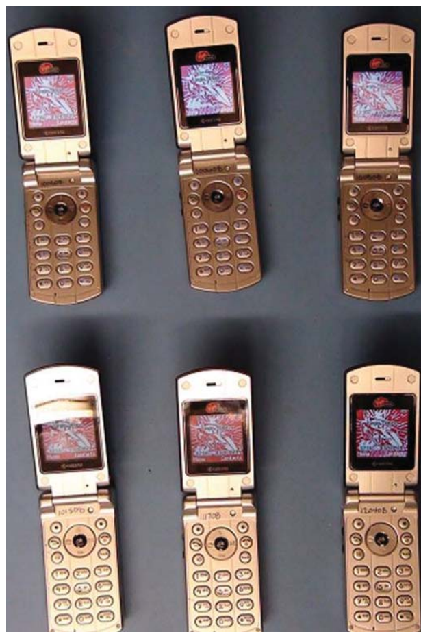
Figure 4-4. Cell phones powered on 12 months after exposure.
