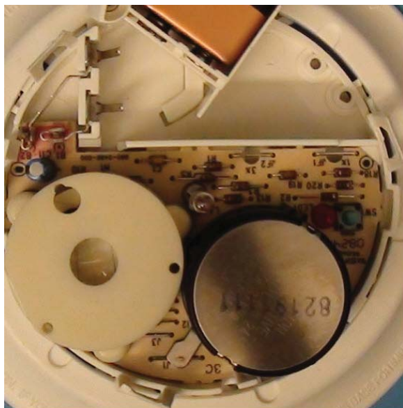
Figure 4-2. (a) Category 2 metals, (b) Inside of a smoke detector, and (c) exposed wire of stranded wire 12 months after H_2O_2 fumigation.
