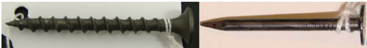
Figure 3-2. (a) Stranded wire, DSL conditioner, and steel outlet/switch box with sealant (caulk), (b) gasket and (c) drywall screws and nails used in the compatibility testing.
